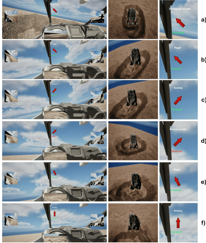
Figure 9: Step-by-step evaluation of LMM-assisted recovery from being stuck in scenario 8. The figure shows a top-down view of the flow of advisory instructions followed. The left column entails the driver's view, the middle column view, unavailable to the driver, is a bird's-eye view for demonstration purposes only, and the right column is an enlarged representation of LMM instructions. a) The vehicle's initial position is inside the uphill entrapment ditch. LMM guides the driver for leftward steering with directional escape behavior and forward throttle. Through these assisted instructions, the driver attempts to climb up the steep hill. b) In addition to the previous step, to gain more traction through the contact patch, LMM instructs wiggle movement in the forward direction for lateral wheel displacement. c) Despite the previous inputs, the vehicle cannot gain traction for further left-forward direction movement. As a result, LMM instructs the driver to rock the throttle in a right-forward direction to gain traction through a jerking movement. d) With no significant movement achieved, LMM adapts to the situation and instructs the driver to reverse while steering right, allowing the vehicle to attempt to align in a different, more favorable direction. e) After sufficient vehicle reverse movement, LMM instructs in forward wiggle movement while steering left, allowing the vehicle's rear wheels to approach the entrapment edge. f) Finally, while maintaining momentum, the LMM assists the driver in applying the throttle in a rocking pattern while steering straight. This results in a sudden gain in traction, ultimately allowing the vehicle to recover from the stuck situation.
