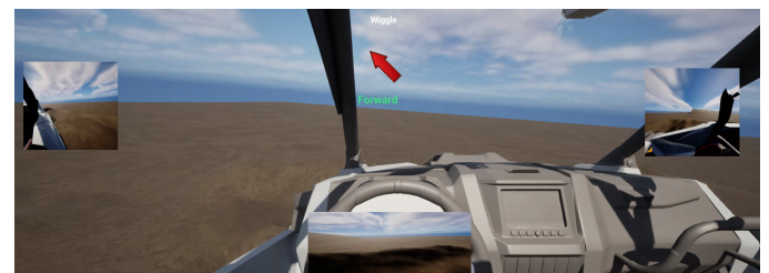
Figure 3: Driver-facing HMI portraying a simulated off-road vehicle cockpit. The display features lateral, forward, and backward views, and the UI supports LMM-assisted instructions with arrows for direction, forward/reverse movement, and maneuver behavior.
